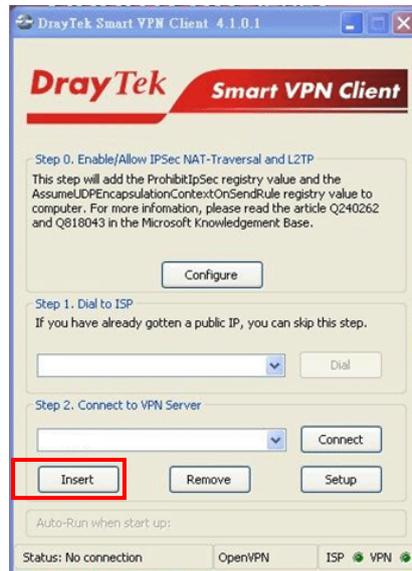
2. Type a name (e.g., Profile 6) as the **Profile Name** and an IP address (e.g., 200.200.200.200) as VPN Server IP. Set jos/jos as the **User Name/Password**. Click **OpenVPN** as the type of VPN and click **OK** to display the **OpenVPN Setting** dialog.
