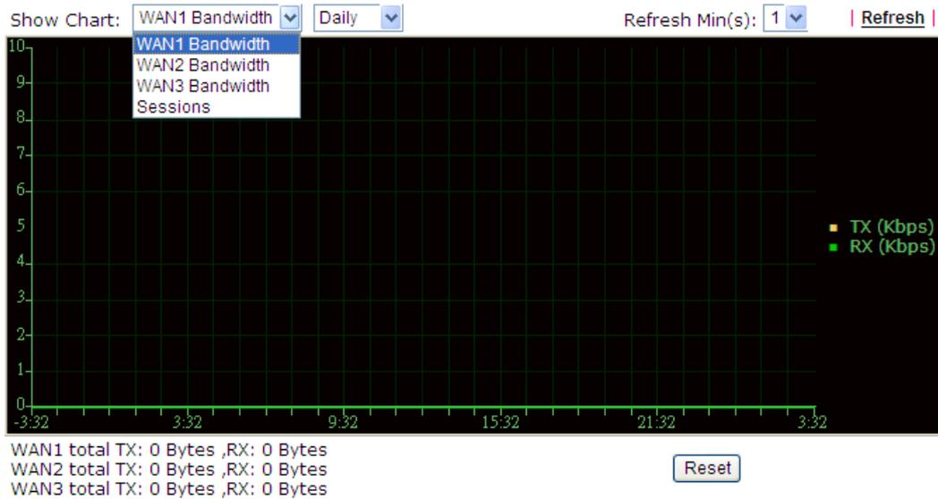
The horizontal axis represents time. Yet the vertical axis has different meanings. For WAN1/WAN2/WAN3 Bandwidth chart, the numbers displayed on vertical axis represent the numbers of the transmitted and received packets in the past.
